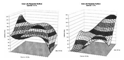
The results of the combined optimizations led to over a 20 times improvement in lifetime when compared to the unstabilized PC dyes.
